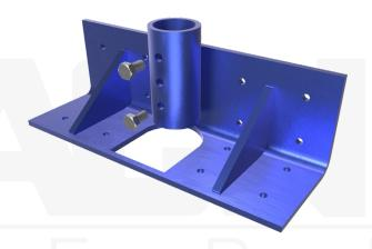
**Installation Notes:** Prepare the existing foundation. Core a 3.50" diameter or larger hole through the footing or slab where the push pier is located. Attach the bracket and MAGNUM® ram. Install the push pier through the core hole to the required pressure and load test. Lift the structure as needed using either a MAGNUM® ram or lifting fixture. Drill holes and bolt the bracket to the pile. (Expansion Anchors Sold Separately)
