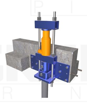
**Installation Notes:** After installation of pier and bracket, attach lifting assembly (MP1008A-3) to the bracket underside using the bolt provided. Snug tighten nuts on top fixture. Attach second top fixture (MP1008B-3). Place a hydraulic power pack or bottle jack between the top fixtures and lift as required. Re-tighten nuts to secure pile and bracket position. Remove upper fixture (MP1008B-3) and re-use on other piles.
