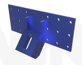
**Installation Notes:** Prepare the existing foundation. Install the helical anchor to the correct depth and torque. Install a MAGNUM® MHC1080 pile cap on the anchor. Mount the bracket by sliding down over the thread bar into position. Secure to the anchor and post-tension as required for the project. Use spherical or wedge washer if anchor is not sufficiently perpendicular to bearing plate. (Expansion Anchors Sold Separately)
