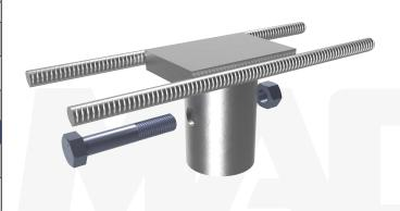
**Notes:** Cap capacity is developed using the ASD design method and considers strength of collar, end effecter, and pile connection. Capacity may be limited by the helical pile, bearing/pullout capacity of soil, or strength of the concrete the cap is embedded in.
