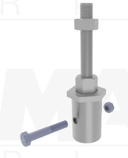
Installation Notes: After installation of a MAGNUM® Helical pile and any extensions, place the cap on the last segment and secure with (1) 7/8" bolt, snug tighten nut. Omit the thread bar, and continue installation until the correct depth and torque is achieved. Install the thread bar and bearing plate, whalers or brackets as applicable. Snug tighten or posttension thread bar nut against bearing plate as required for the project.
