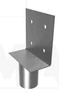
Installation Notes: After installation of a MAGNUM® Helical Pile to the correct depth, torque, and capacity, cut-off the pile shaft at the proper elevation. Place the pile cap over the shaft and secure with 4 Hilti EDS PAF. Place wood beam on cap angle and secure with 1/2" lag bolts as required for the project. If required, install MAGNUM® K-brace system in accordance with installation instructions for that product.
