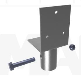
Installation Notes: After installation of a MAGNUM® Helical Pile to the correct depth, torque, and capacity, cut-off the pile shaft at the proper elevation. Drill (1) 15/16" diameter hole through the shaft using a MAGNUM® drill template. Place the pile cap over the shaft and secure with (1) 7/8" bolt. Snug tighten nut. Place wood beam on cap angle and secure with 1/2" lag bolts as required for the project.
