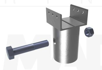
Installation Notes: After installation of a MAGNUM® Helical Pile to the correct depth, torque, and capacity, cut-off the pile shaft at the proper elevation. Drill 1-1/16" hole using a MAGNUM® drill template. Place the pile cap over the shaft and secure with (1) 1" bolt. Snug tighten nut. Place wood post on post base and secure with 1/4" lag bolts as required for the project.
