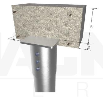
Installation Notes: After installation of a MAGNUM® Helical Pile to the correct depth, torque, and capacity, cut-off the pile shaft at the proper elevation. Drill (3) 1-9/16" diameter holes through the shaft using a MAGNUM® drill template, place the cap over the shaft and secure with (3) 1-1/2" bolts. Snug tighten nut. Ensure direct bearing of plate on shaft. Place reinforcing steel, cast concrete and consolidate around the pile cap per project requirements.
