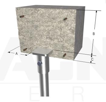
Installation Notes: After installation of a MAGNUM® Helical Pile to the correct depth, torque, and capacity, cut-off the pile shaft at the proper elevation. Drill (1) 1-5/16" diameter hole through the shaft using a MAGNUM® drill template, place the cap over the shaft and secure with (1) 1-1/4" bolt. Snug tighten nut. Ensure direct bearing of plate on shaft. Place reinforcing steel, cast concrete and consolidate around the pile cap per project requirements.
