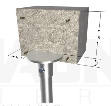
Installation Notes: After installation of a MAGNUM® Helical Pile to the correct depth, torque, and capacity, cut-off the pile shaft at the proper elevation. Drill (1) 1-9/16" diameter hole through the shaft using a MAGNUM® drill template, place the cap over the shaft and secure with (1) 1-1/2" bolt. Snug tighten nut. Ensure direct bearing of plate on shaft. Place reinforcing steel, cast concrete and consolidate around the pile cap per project requirements.
