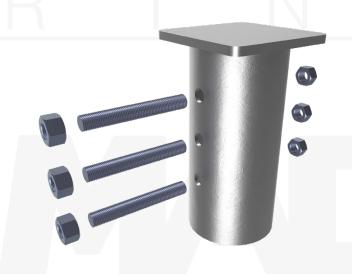
Installation Notes: After installation of a MAGNUM® Helical Pile to the correct depth, torque, and capacity, cut-off the pile shaft at the proper elevation. Drill (3) 1-9/16" diameter holes through the shaft using a MAGNUM® drill template, place the cap over the shaft and secure with (3) 1-1/2" bolts. Snug tighten nut. Ensure direct bearing of plate on shaft. Place reinforcing steel, cast concrete and consolidate around the pile cap per project requirements.
