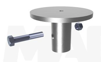
Installation Notes: After installation of a MAGNUM® Helical Pile to the correct depth, torque, and capacity, cut-off the pile shaft at the proper elevation. Drill (1) 1-1/16" hole through the shaft using a MAGNUM® drill template. Place the pile cap over the shaft and secure with (1) 1" bolt. Snug tighten nut. Alternatively, drilling through pile may be omitted and plug welds may be used to secure cap to pile in place of bolts, see MAGNUM® Technical Bulletin TB004.
