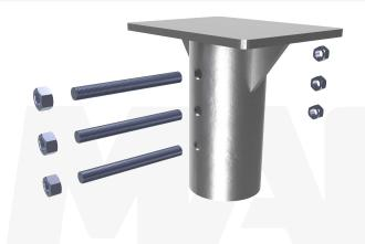
Installation Notes: After installation of a MAGNUM® Helical Pile to the correct depth, torque, and capacity, cut-off the pile shaft at the proper elevation. Drill (3) 1-9/16" holes through the shaft using a MAGNUM® drill template, place the cap over the shaft and secure with (3) 1-1/2" bolts. Snug tighten nuts. Alternatively, drilling through pile may be omitted and plug welds may be used to secure cap to pile in place of bolt(s), see MAGNUM® Technical Bulletin TB004.
