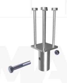
**Notes:** Cap capacity is developed using the ASD design method and considers strength of collar, end effecter, and pile connection. Rebar studs conform to ACI 318 dimensions and are designed to have full tension development in normal weight concrete with 28-day f'c  $\geq$  3,000 psi. Capacity may be limited by the helical pile, bearing/pullout capacity of soil, or strength of the concrete the cap is embedded in.
