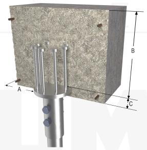
A - As Required for Shear (Min. 4" per IBC)
