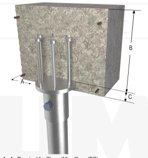
A - As Required for Shear (Min. 4" per IBC)
