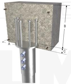
A - As Required for Shear (Min. 4" per IBC)
