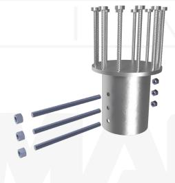
**Notes:** Cap capacity is developed using the ASD design method and considers strength of collar, end effecter, and pile connection. Rebar studs conform to ACI 318 dimensions and are designed to have full tension development in normal weight concrete with 28-day f'c  $\geq$  3,000 psi. Capacity may be limited by the helical pile, bearing/pullout capacity of soil, or strength of the concrete the cap is embedded in.
