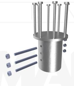
**Notes:** Cap capacity is developed using the ASD design method and considers strength of collar, end effecter, and pile connection. Rebar studs conform to ACI 318 dimensions and are designed to have full tension development in normal weight concrete with 28-day f'c  $\geq$  3,000 psi. Capacity may be limited by the helical pile, bearing/pullout capacity of soil, or strength of the concrete the cap is embedded in.
