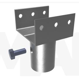
Installation Notes: Protectpile capand boltfrom weather prior to installation. After installation of a MAGNUM® Helical Pile to the correct depth, torque, and capacity, cut-off the pile shaft square at the proper elevation. Place the pile cap over the shaft and secure with (1) 3/4"-16 bolt. Ensure direct bearing of post base on shaft. Tighten bolt to a minimum torque of 50 ft-lbs. Do not exceed 60 ft-lbs. Place wood post and fasten with 1/2" lag screws.
