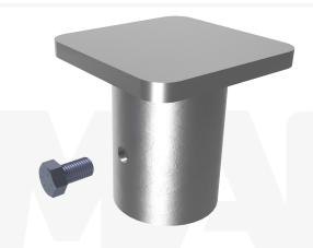
**Installation Notes:** After installation of a MAGNUM® Helical Pile to the correct depth, torque, and capacity, cut-off the pile shaft at the proper elevation. Place the cap over the shaft and secure with (1) 3/4" fine thread bolt. Tighten to specified torque. Ensure direct bearing of plate on shaft. Place reinforcing steel, cast concrete and consolidate around the pile cap per project requirements.
