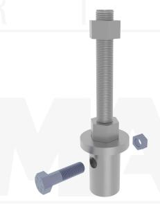
Installation Notes: After installation of a MAGNUM® Helical Anchor or Piers to the correct depth, torque, and capacity, begin by cutting-off the pile shaft at the proper elevation. Drill (1) 1-1/16" hole using the MAGNUM® drill template. Place the pile cap over the shaft and secure with (1) 1" bolt. Snug tighten nuts. Snug tighten or post-tension thread bar nut against bearing plate as required for the project.
