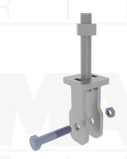
Installation Notes: After installation of the MAGNUM® Helical Pile to the correct, depth, torque and capacity, cut off the pile shaft at the proper elevation. Drill (1) 1-1/16" diameter hole through the shaft using a MAGNUM® drill template. Place the anchor cap over the shaft and secure with (1) 1" bolt. Snug tighten nut. Pass thread bar with nut through the hole in the end plate and make necessary attachments.
