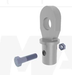
Installation Notes: After installation of a MAGNUM® Helical Pile to the correct, depth, torque and capacity, cut-off the pile shaft at the proper elevation. Drill (1) 1-1/16" diameter holes through the shaft using a MAGNUM® drill template. Place the pile cap over the shaft and secure with (1) 1" bolts. Snug tighten nuts. Alternatively, drilling through pile may be omitted and plug welds may be used to secure cap to pile in place of bolt, see MAGNUM® Technical Bulletin TB004.
